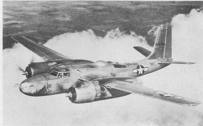
A-26 Invader; with an all-purpose nose allowing complete interchangeability of armament to adapt the plane to various missions.
