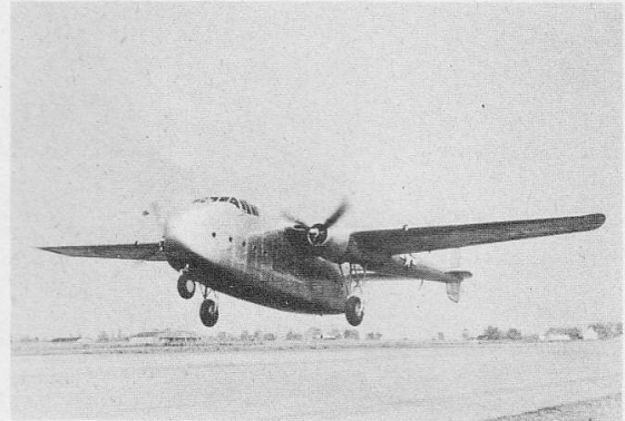
C-82 Packet; called the "Flying Boxcar" because it can carry heavy and bulky equipment.
